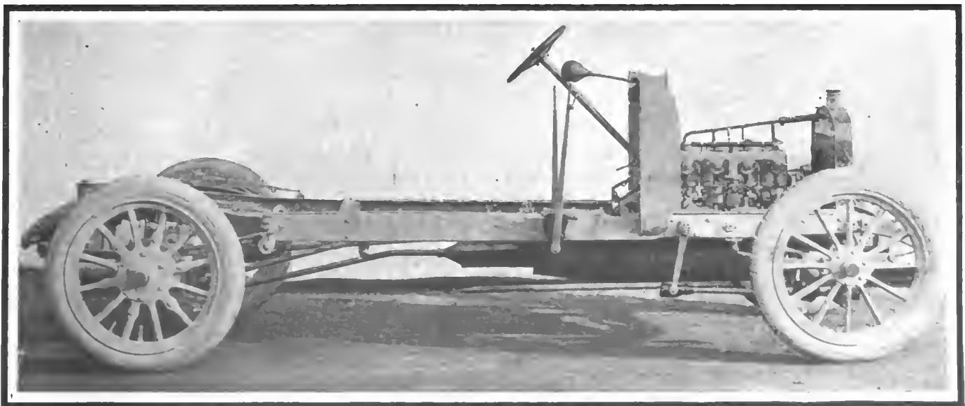
Chassis of the 15-horsepower Austin, showing separate cylinders and cased-in change-speed bracket
